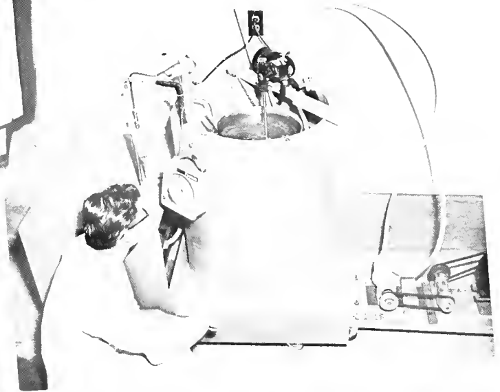
Below. This laboratory refrigeration unit is used to cool a salt-glucose solution for immersion freezing of fish and shellfish.
